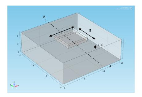
Figure 1.Graphical representation of a soak-away rain garden in COMSOL Multiphysics.
