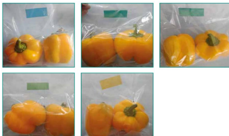
Figure 1. Colour changing of CO 2 indicator [48].
