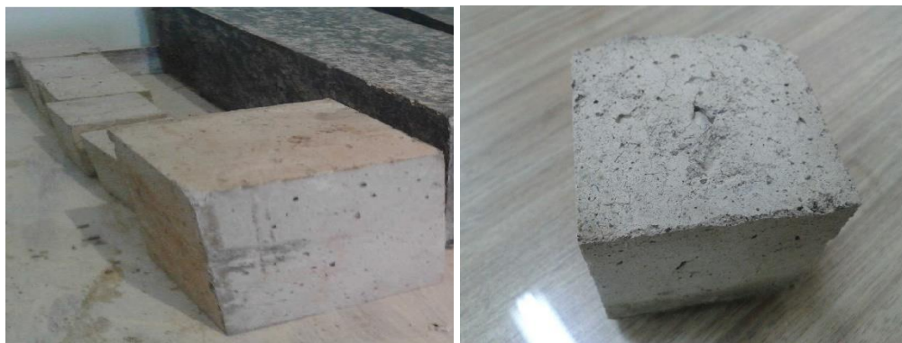
Figure 2. Samples made of geopolymer concrete based on bentonite
