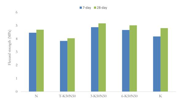
Figure 5. 7-day and 28-day flexural strengths GPC specimens
