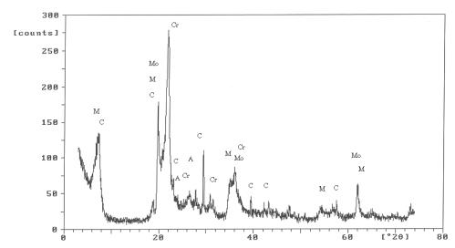
**Figure 1.** X-ray diffraction pattern of the studied bentonite sample and identified phases: Cr; Cristobalite, M; Montmorillonite, C; calcite, Mo; muscovite, A; albite
