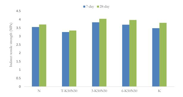
Figure 4. 7-day and 28-day tensile strengths GPC specimens
