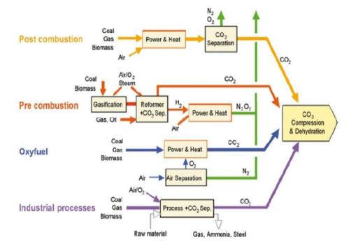
Figure 3. Schematic representation of capture systems [23]
