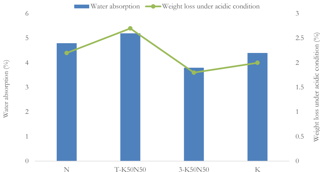
Figure 8. Water absorption and weight loss under acidic conditions of N, T-K50N50, 3-K50N50, and K mixes
